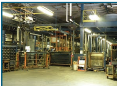
Dixie Industrial Finishing operates five automated plating lines, including large part size capacity tanks (13 feet long X 5 feet deep X 34 inches wide) that allow efficient processing of parts.
